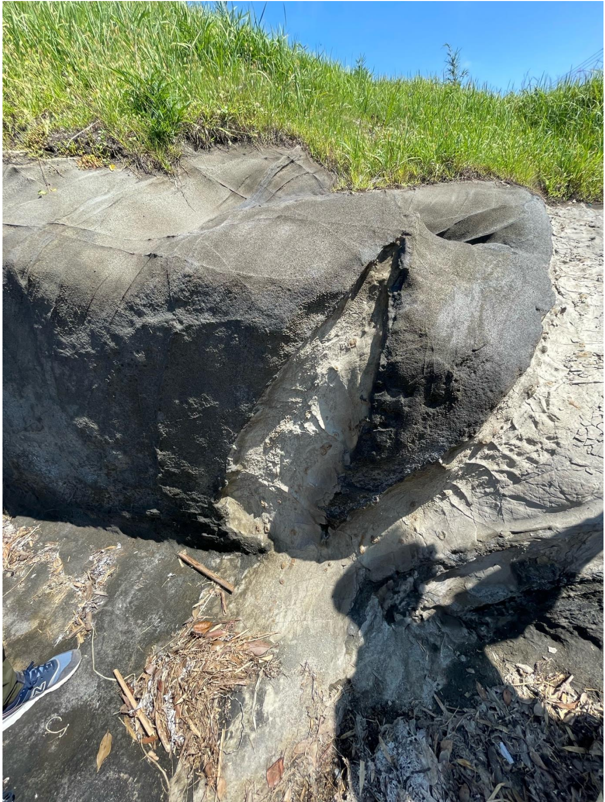
Figure 6. Embedded clast behaving like a weak block within its deforming matrix.
