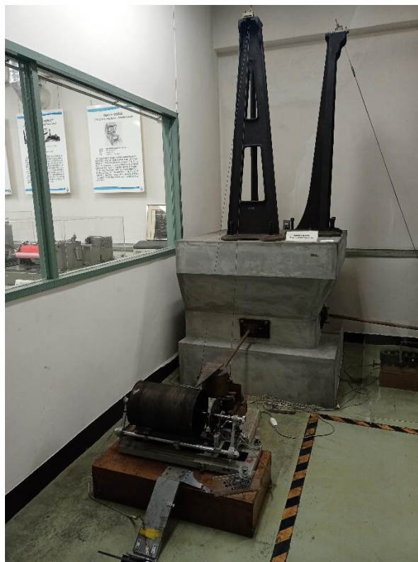
Figure 2. Omori Long Period Seismograph exhibited in Seismograph Museum of ERI
